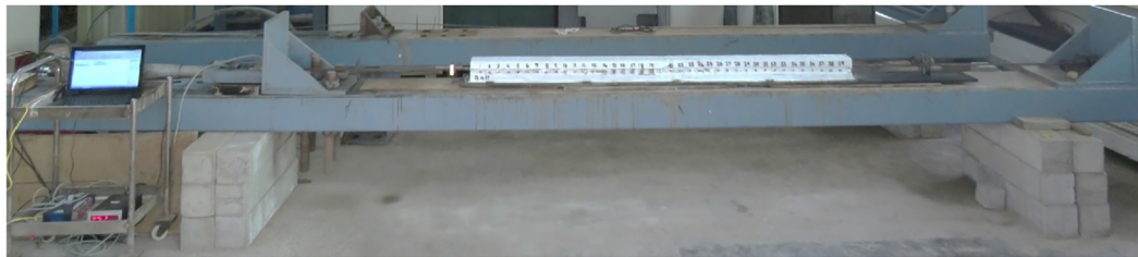
Fig. 5. Sketches and photograph of prestressing bed with PTC specimen.
